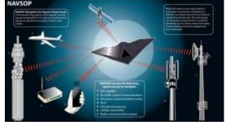
tricks a device into misidentifying its location. The new system can learn from signals that are initially unidentified to build an ever more accurate and reliable fix on its location. Even the signals from GPS jammers can be exploited by the device to aid navigation under certain conditions.
