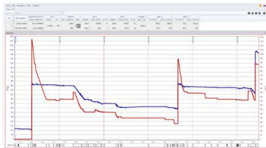
Fig. 3: Fuel level graph comparing the readings from a standard fuel sensor (red) and the Escort fuel level sensor (blue)
