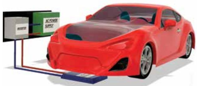
3D Model of Magnetically Coupled Static Wireless Charging System
