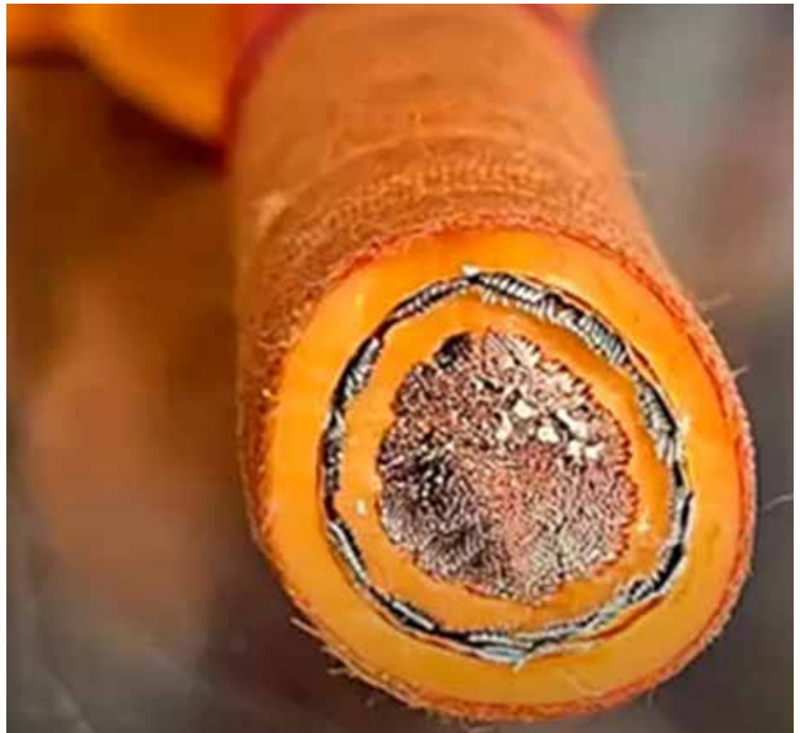
Figure 1 : Cross-Sectional View of a Tesla Supply Interconnect Cable
