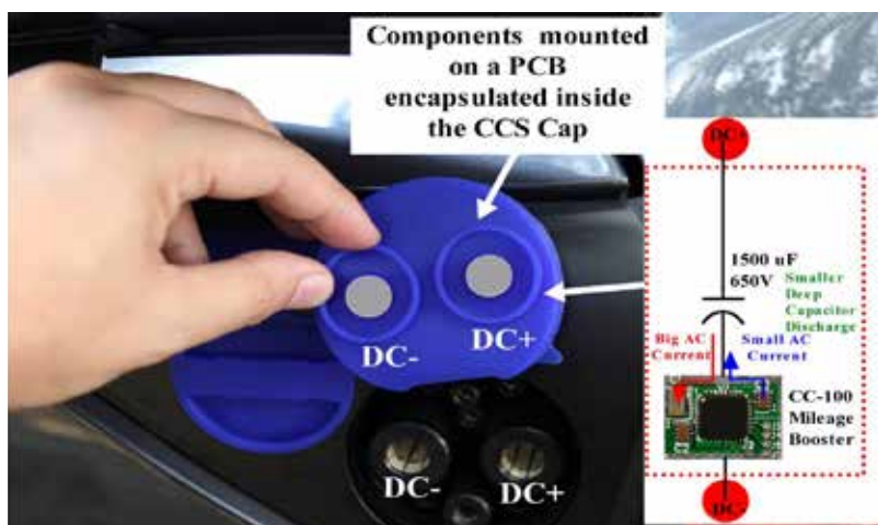
Figure 5 : CC-100 Enhanced DC-Link Capacitor Embedded in a Charging Port CCS Cap
